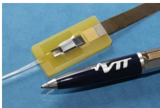
12 \mu\text{m} SOI chip with spot-size converters
